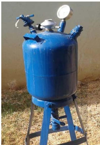
Fig. 1 10-Liter Locally fabricated laboratory scale biodigester
